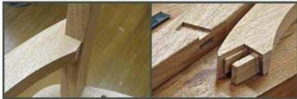
The joint between the armrest plate and the rear legs is a four-sided mortise and tenon joint with dovetail joints on the sides of the rear legs to enhance the joint.
