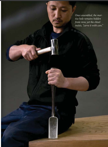
The primary role of the striking chisel is to carve mortise holes, which is why it's built to be durable.
