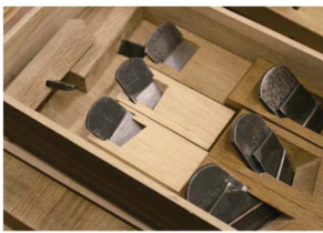
Various types of planes are produced, including one that only carves the edges in the center of the photo.
