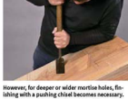
However, for deeper or wider mortise holes, finishing with a pushing chisel becomes necessary.
